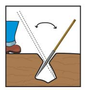
(1) Insert the dibble bar or other tool straight into the ground, pull backward on the handle and push forward to make a small hole.
