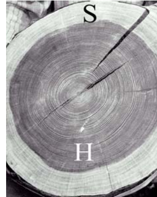
Figure 2. Cross-section of log showing heartwood (H) and sapwood (S).
