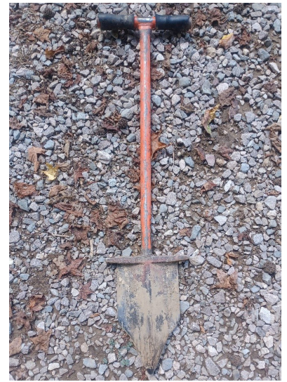
Figure 5: RA KBC bar modified to increase width of the planting bar to facilitate planting larger size seedlings. Photo Courtesy: Stacy Clark, USDA Forest Service.
