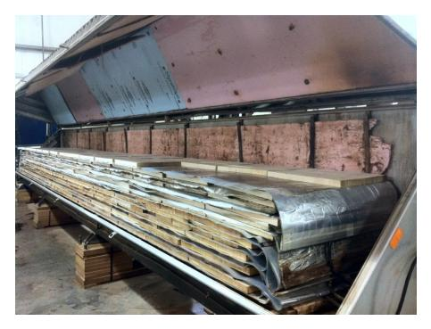
*Figure 2.* This clamshell-like vacuum kiln is used to dry high-value hardwood blanks for a guitar factory. The silvery pieces of fabric are used to heat the wood.
