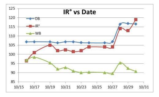
**Figure 17.** Data from a commercial DH kiln run with hickory sapwood. The surface temperature readings taken with a handheld infrared thermometer approached the dry bulb temperature on October  $24^{th}$ . DB= dry bulb temperature (°F), WB = wet bulb temperature (°F), and IR° = the infrared thermometer reading (°F). The IR thermometer readings aren't as precise as the kiln temperature readings, and so they appear to vary more than the kiln temperature readings.
