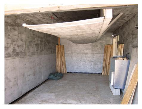
**Figure 4.** In this DH kiln the compressor unit is to the right. The hinged piece of plywood near the ceiling is a baffle that drops to direct circulating air through the stacks of lumber. There is a small powered vent at the rear.
