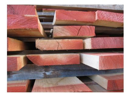
**Figure 35.** A sprayer was used to apply end coat to these oak boards, but the end coating wasn't applied carefully or heavily enough to be very effective. Notice the overspray and the many end checks. The stickers weren't placed close to the board ends either and that would have also helped to minimize the loss due to end checks.
