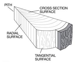
*Figure 11.* This sketch labels the cross section, radial surface and the tangential surface on a wedge of wood.<sup>2</sup>
