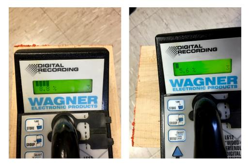
*Figure 46.* Different readings with a dielectric moisture meter on the same (cupped) board. The meter is parallel to the grain in the left-hand photo and turned at 90° to the grain in the right-hand photograph.
