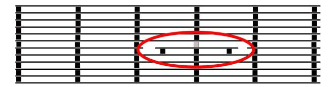
**Figure 42.** This diagram shows a kiln sample pocket in a stack of ten-foot lumber. The gray sticker above the sample board should be shorter than the rest to make it easy to remove and replace the sample board. The stickers supporting the ends of the sample boards can be shorter than the rest.
