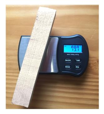
*Figure 18.* Low capacity balance for weighing small moisture sections. This balance weighs to the nearest 0.1 gram and has a capacity of 2.2 pounds (1000 grams).
