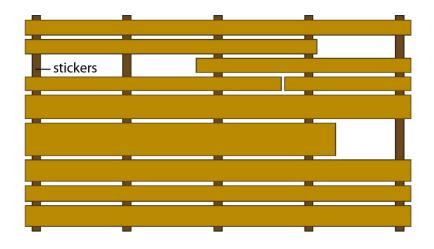
*Figure 39.* This is a top-down view of box piling. Notice the full-length boards placed along the front and back edges of the pile; shorter boards get placed in the middle.
