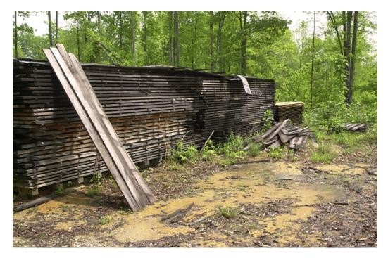
*Figure 34.* This lumber is too close to the ground, vegetation needs to be cleared and the area in front of the stacks collects water. None of this will help a sawmill dry high-quality lumber.
