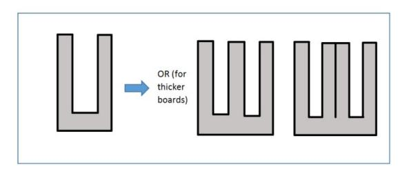
**Figure 27.** A single pair of prongs is appropriate for 4/4 boards, but thicker boards are usually cut somewhat differently. You are looking at representations of the end grain in these diagrams. For 4/4 boards, the prongs should be about one-quarter of the board thickness.
