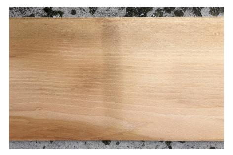
*Figure 38.* The dark stripe in the middle of this board resulted from the contact of the board with a stacking sticker and is commonly called sticker stain or sticker shadow.
