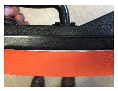
*Figure 47.* Dielectric moisture meters cannot make an accurate reading if the electrode plate can't make full contact because the lumber is cupped. In this photo the meter is perpendicular to the grain.
