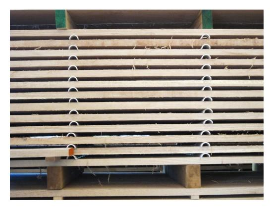
*Figure 37.* Cut 1-1/2" PVC pipe can be used to make light-duty stickers with good air flow characteristics. The stickers should have been better aligned with the bolsters here.
