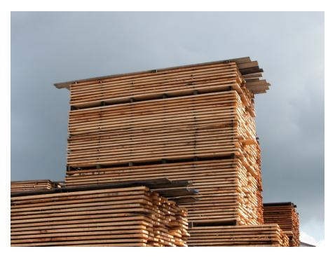
**Figure 33.** This lumber is well stacked and the yard manager has added stack covers (made of weighted-down boards in this case) above the top layer of lumber to protect the lumber. Note the stickers used to keep the stack covers away from the top layer.
