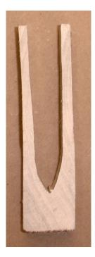
*Figure 9.* In stress-free lumber the prongs will remain straight after the sample has cooled.
