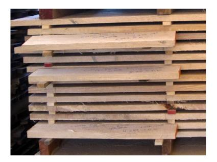
Figure 43. Cantilevered sample boards used for lumber that has been previously air-dried.
