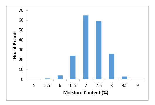
**Figure 24.** A final moisture content distribution similar to this ought to be the goal of every hardwood dry kiln operator. For this illustration, I assumed that the target average moisture content was 7%, with an allowable tolerance of  $\pm$ 1% moisture content. With very few exceptions, the lumber falls within the range of 6-8% moisture content.
