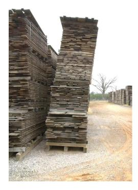
*Figure 45.* Don't position your stacks like this! In spite of the obvious problem with this pile of lumber, this yard has tried to do things right. The piles have stack covers, the yard looks well-drained and free of vegetation, and the lumber is placed on double bunks to raise it off the ground.
