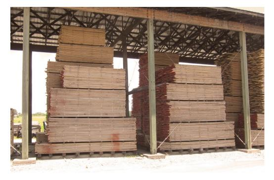
Here's a good example of how to stack air-drying lumber (Figure 32):
