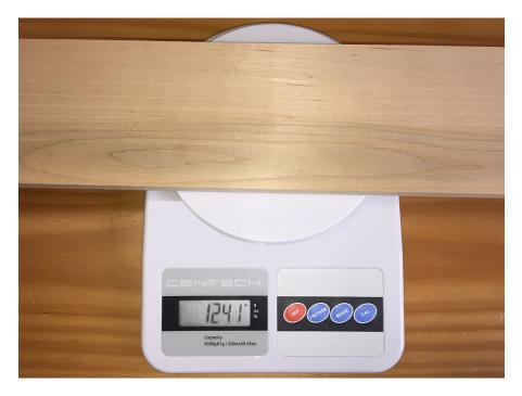
*Figure 19. Higher capacity balance for weighing sample boards. This balance measures to the nearest gram and has an 11 pound (5,000 gram) capacity.*
