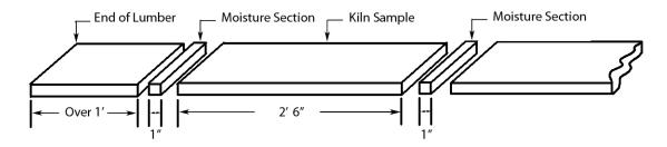
Figure 41. Cut your moisture sections and kiln samples like this. Redrawn from Drying Hardwood Lumber.
