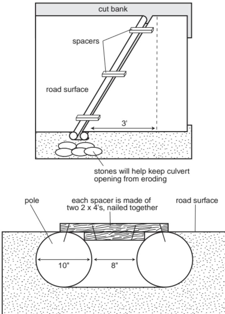
**Figure 1-7–Open-topped Box Culvert**
