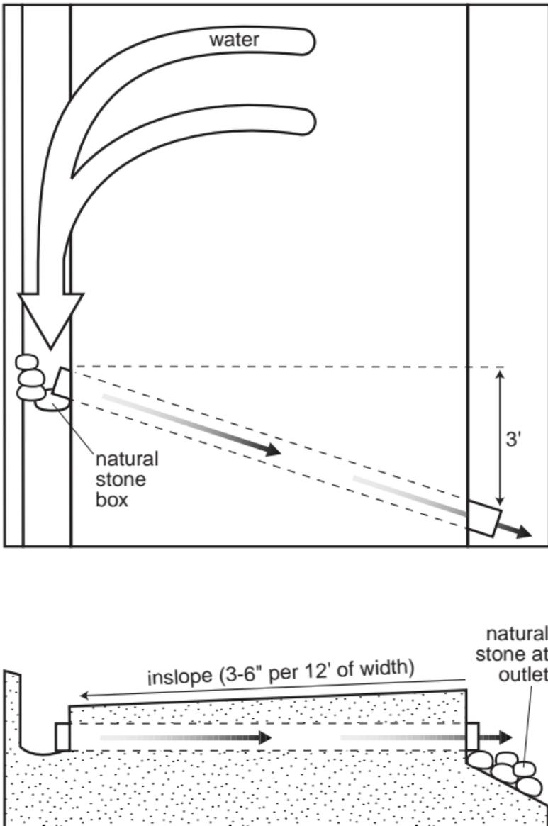
**Pipe Diameter:** Minimum of 12 inches (corrugated metal) or equivalent size double-walled plastic.
